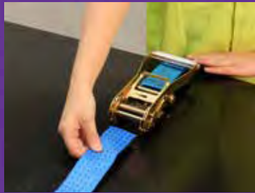
1 Insert loose end of strap into mandrel of ratchet
