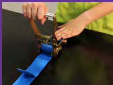
4 Crank the ratchet to desired tightening
