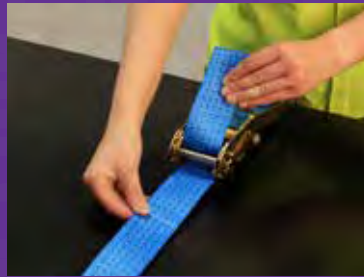
2 Pull strap through slot in mandrel
