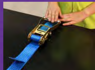
6 Lock handle down after tightening
