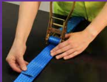
5 Make sure strap stays in line with other to avoid tangling/locking
