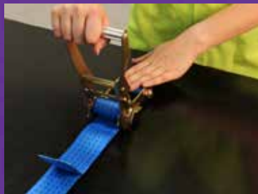
4 Crank the ratchet to desired tightening
