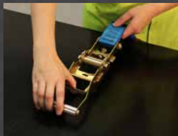
5 Pull trigger to unlock
