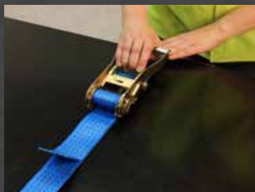
1 Pull trigger toward back handle
